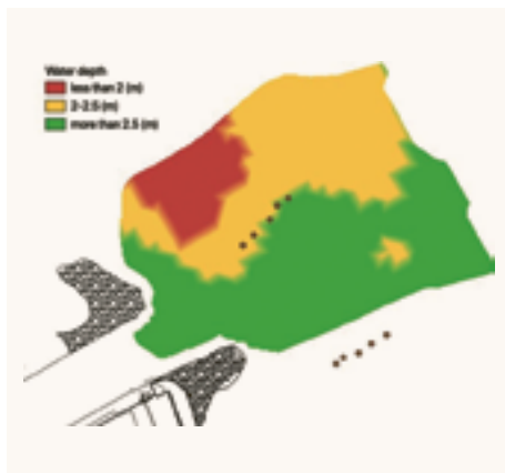
FIGURE 6 Colormap of water depth for specific ranges (more than 3 m, between 2–2.5 m and lower than 2 m) on 30 April 2020. The red circles indicate the GPS reference of the mooring points of inlet and outlet ejectors pipelines. The ejectors are installed between the inlet/outlet mooring points, as shown in Figure 2.
