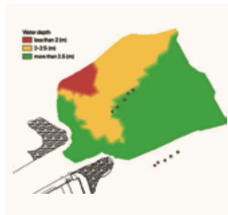
FIGURE 7 Colormap of water depth for specific ranges (more than 3.0 m, between 2.0–2.5 m and lower than 2.0 m) on 11 September 2020. The red circles indicate the GPS reference of the mooring points of inlet and outlet ejectors pipelines. The ejectors are installed between the inlet/outlet mooring points, as shown in Figure 2.
