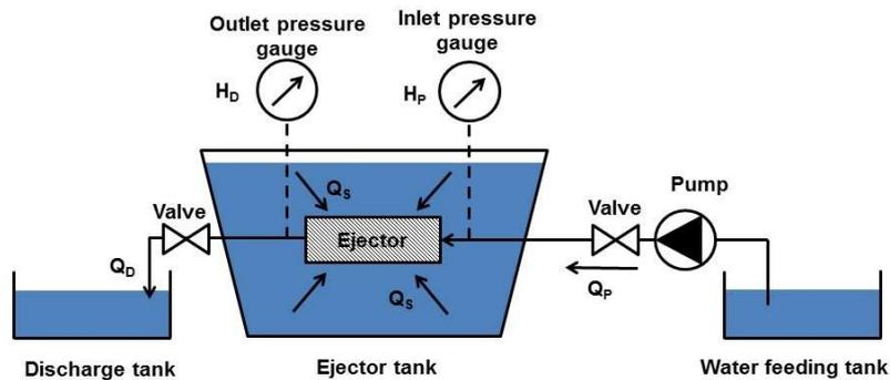
Figure 8. Laboratory testing equipment for ejectors.
