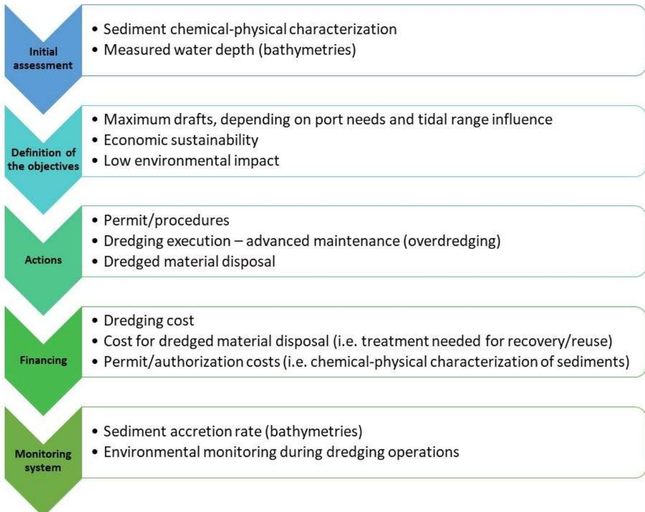
Figure 1. Schematization of a maintenance dredging plan.
