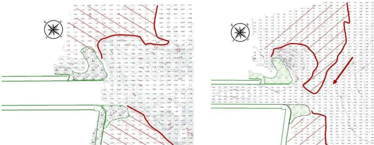
Figure 6. Example of bathymetry analysis: on the left the bathymetries after sediment handling through propellers (May 2009), on the right the bathymetries seven months later (December 2009). The red line indicates the – 2.00 meters of water depth.
