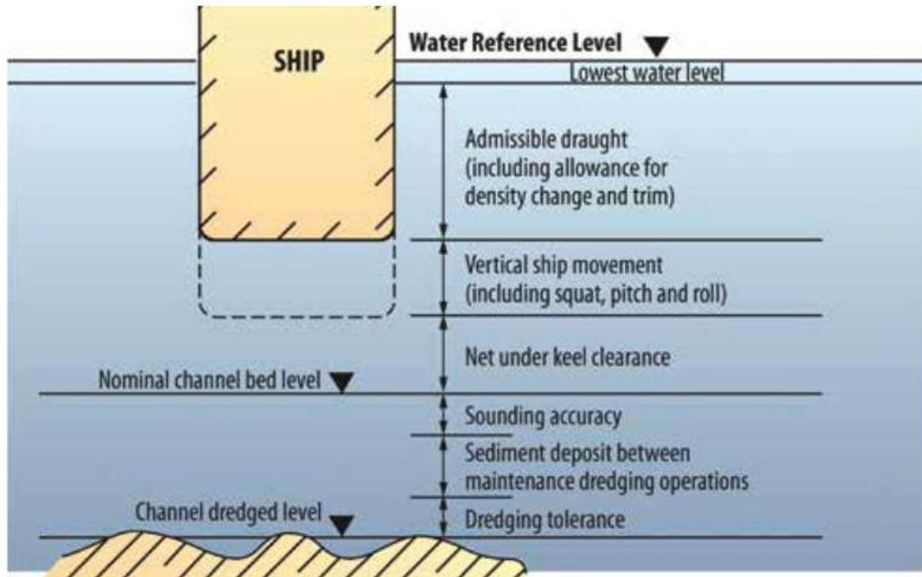
Figure 2. Components of water depth design.
