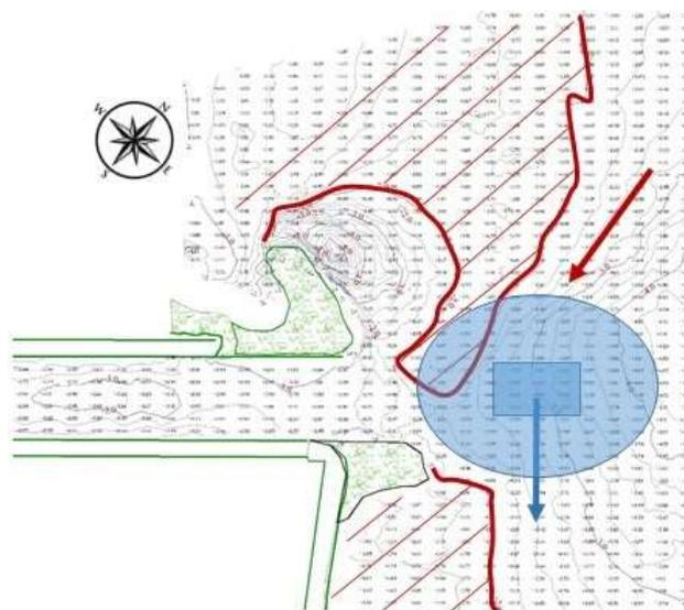
Figure 7. The expected impact of the demo plant on natural sediment transport.
