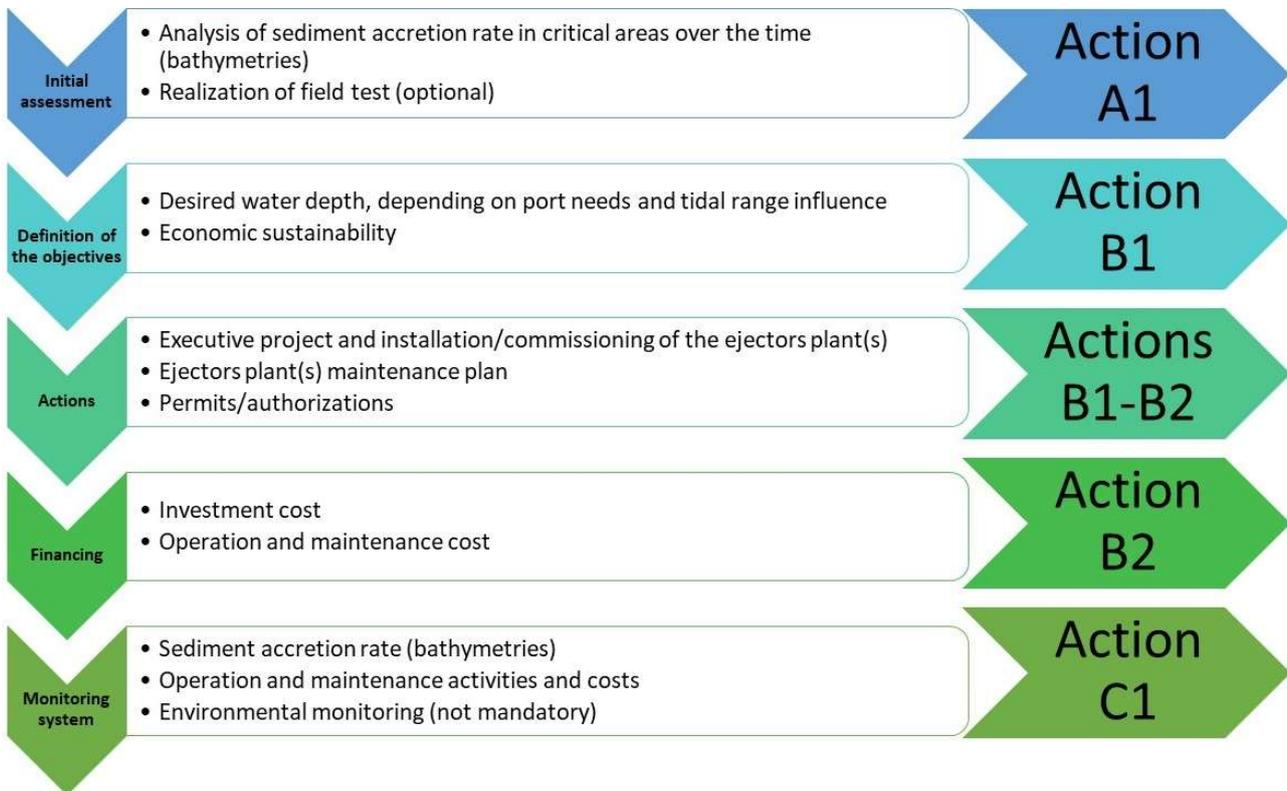
Figure 4. Structure of the seabed maintenance management plan and relation with LIFE MARINAPLAN PLUS project Actions.
