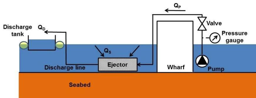
Figure 9. Field testing equipment for ejectors.
