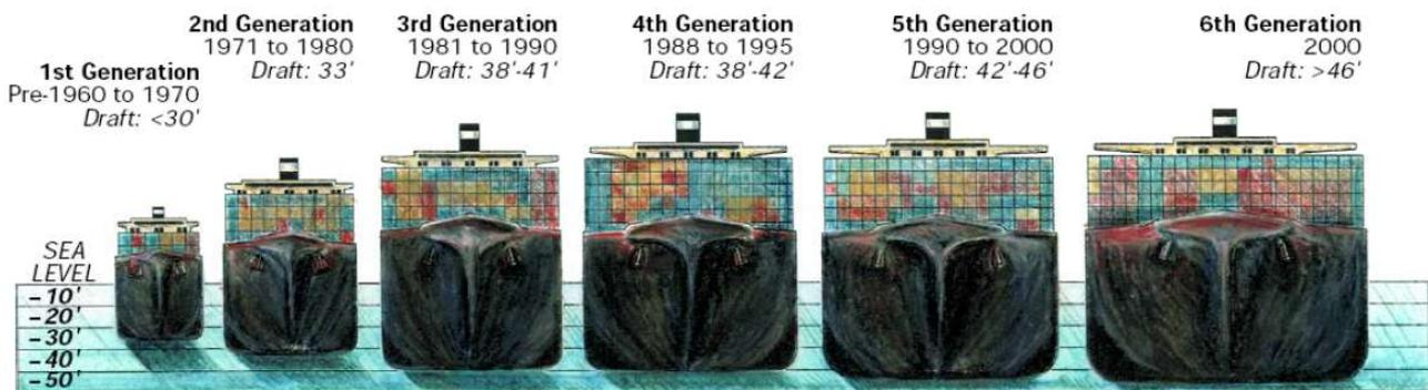
Figure 3. Evolution of loaded cargo draft.
